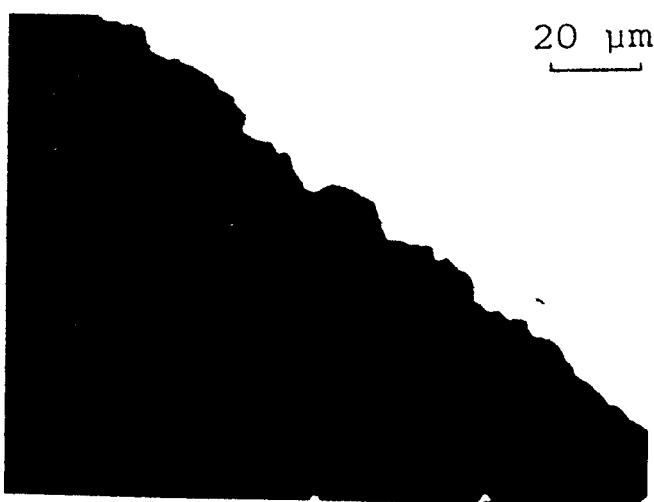
FIG. 1. Optical micrograph of a portion of a polished section of an Sn-YBa 2 Cu 3 O 7-δ -Sn three-layer composite containing 33.3 vol. % Sn. The bright region is tin; the dark region is YBa 2 Cu 3 O 7-δ .
